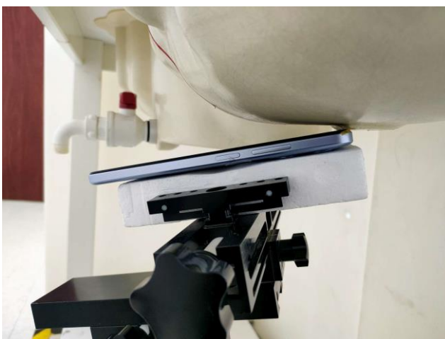
Left Tilted, Test Separation 0 mm
