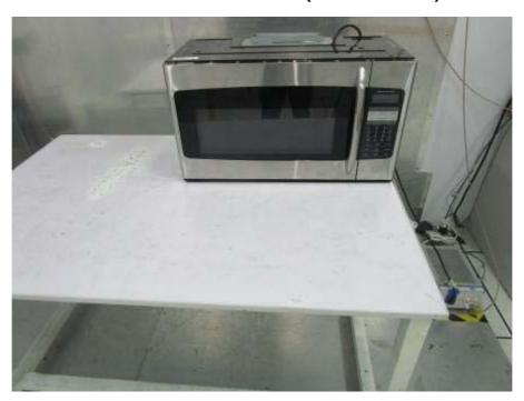
1.2 Radiated Emissions (30MHz-1GHz) Test Setup
