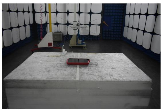
3. Radiated emission (9KHz-30MHz)
