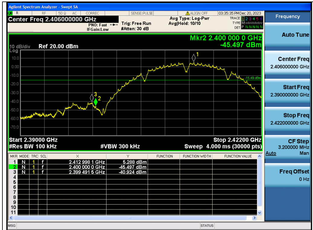
Test_Graph_802.11b_ANT1_2412_1Mbps_Lower Band Edge Emissions
