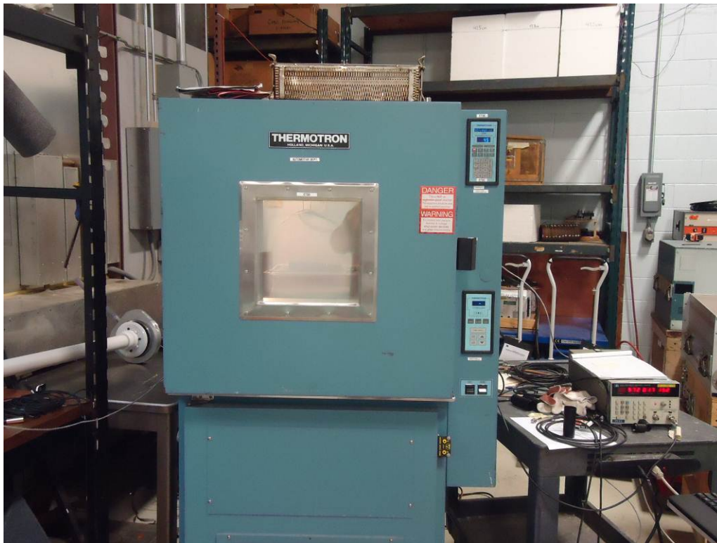
Test Setup for Frequency Stability Test
