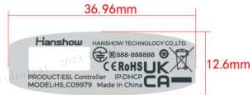
Figure 2-1 Nameplate of HS_C09979
