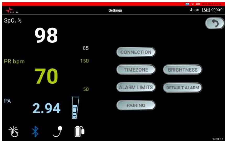
NOTE: Alarm limits can be adjusted only when the Oximeter Box has been paired.
