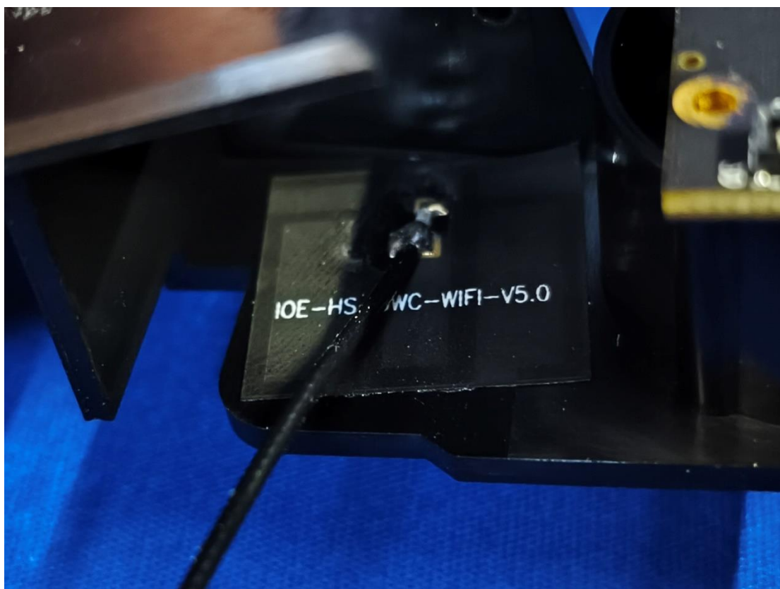
WiFi antenna 2+BT antenna
