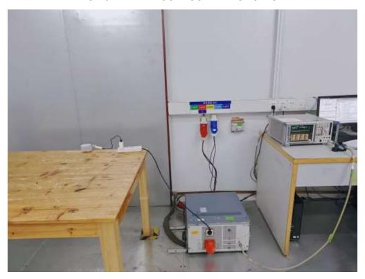
RF CONDUCTED TEST SETUP
