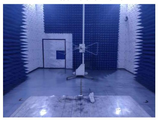
RADIATED EMISSION TEST SETUP ABOVE 1GHz
