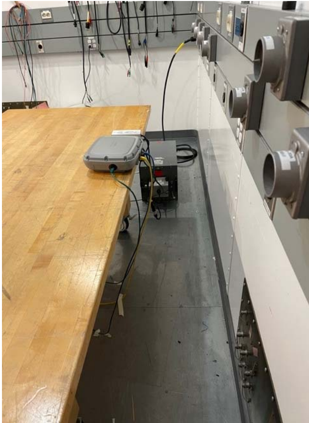
Title: AC Conducted Emissions Test Setup
