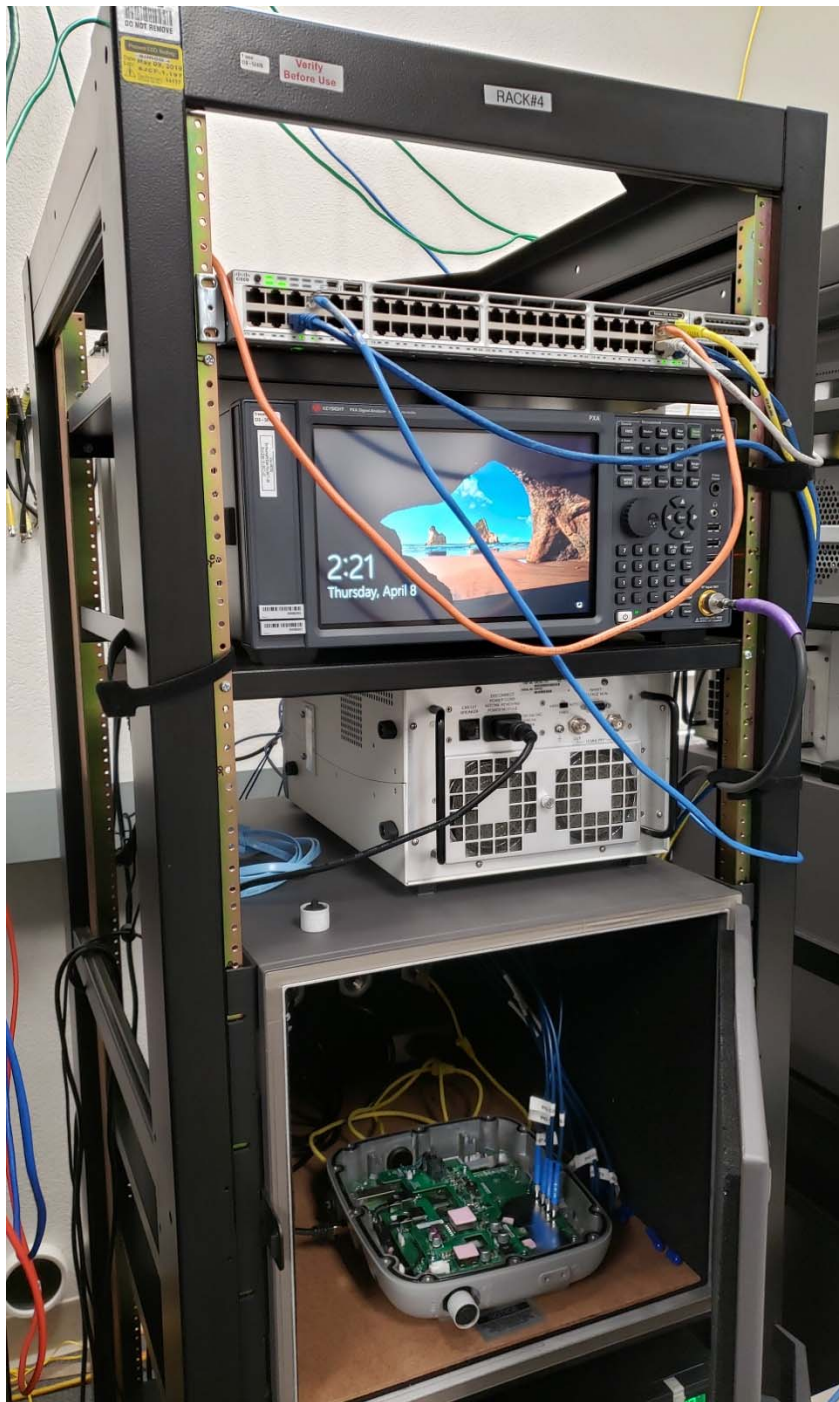
Title: Radio Conducted Test Setup – Rack 4
