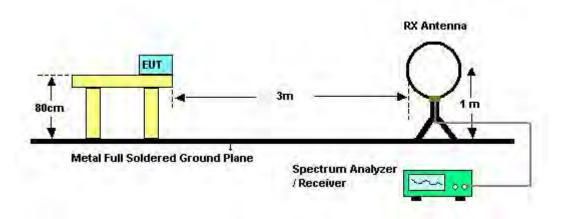
For Radiated Emissions: 30MHz~1GHz
