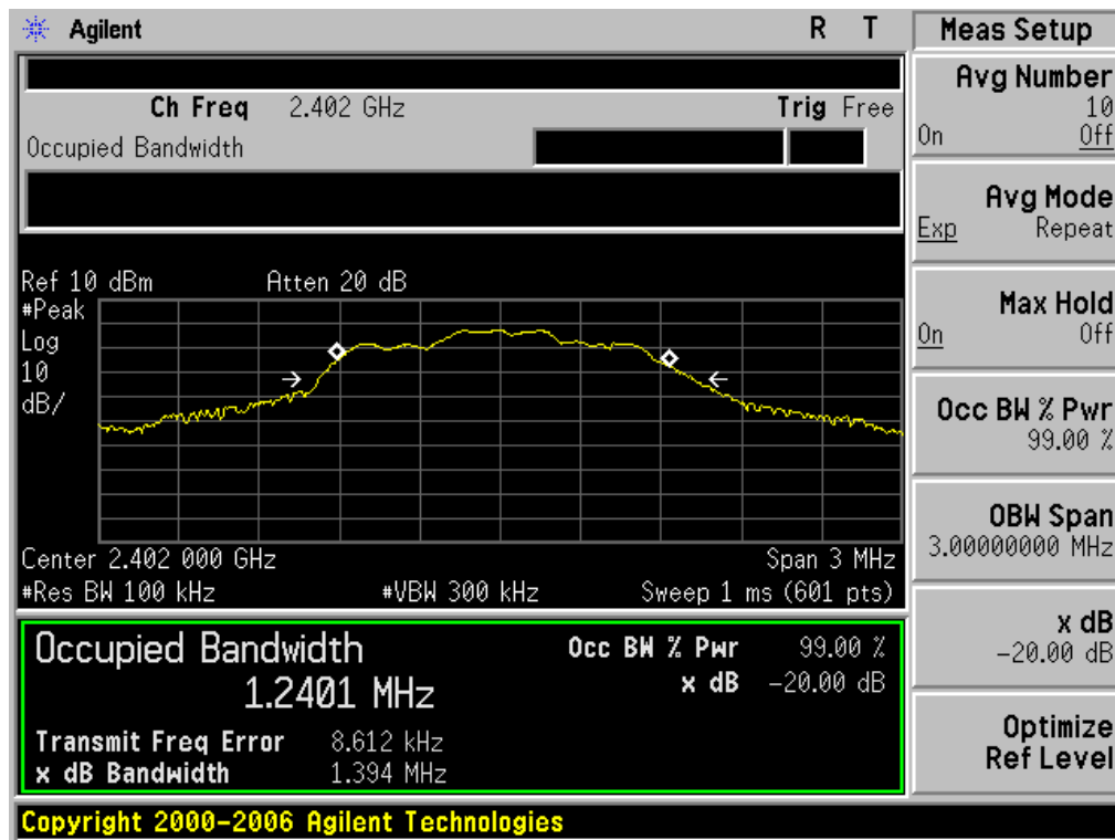
TEST PLOT OF BANDWIDTH FOR LOW CHANNEL
