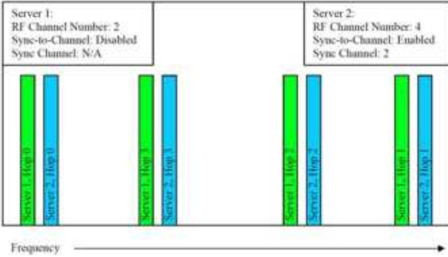
Figure 8: Two servers with Sync to Channel enabled
