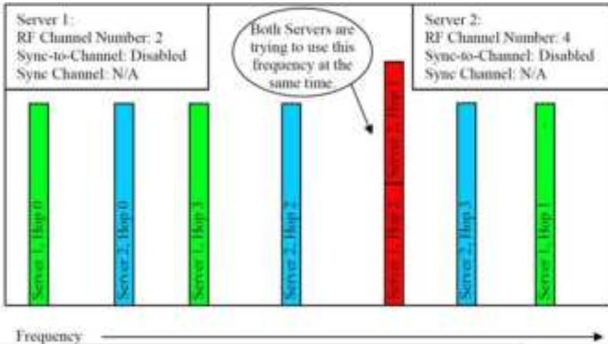
**Figure 7: Two servers without Sync to Channel enabled**
