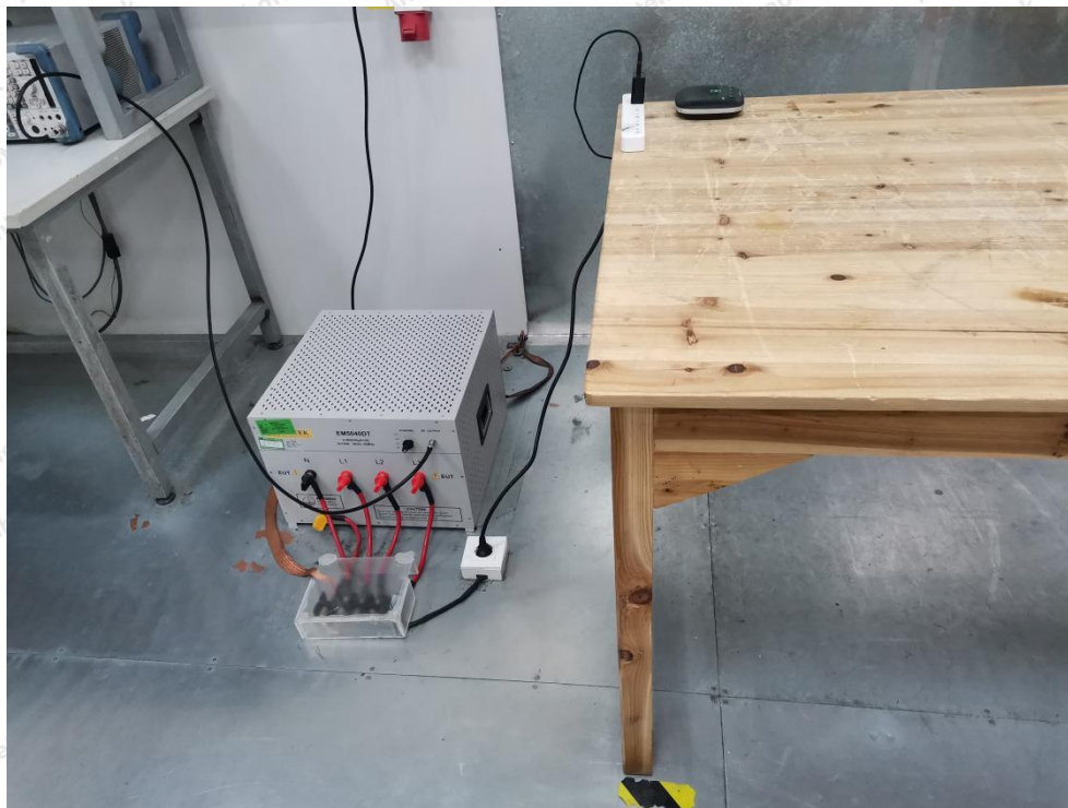
Photo of Conducted Emission Measurement
