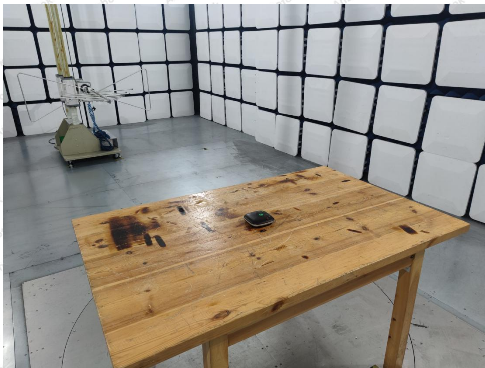
Photo of Radiation Emission Test
