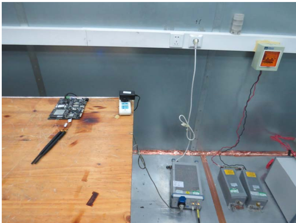
Picture 2 Conducted Emission Test Setup
