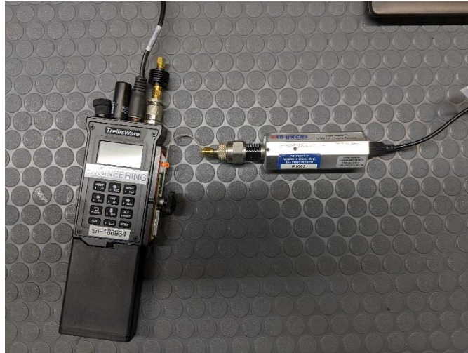
Figure 9 – Test setup, antenna conducted port: power measurement.
