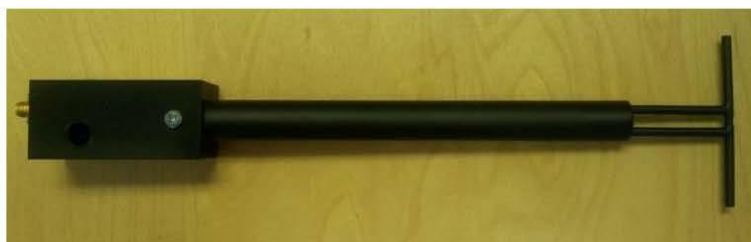
Figure 1 – MVG COMOSAR Validation Dipole
