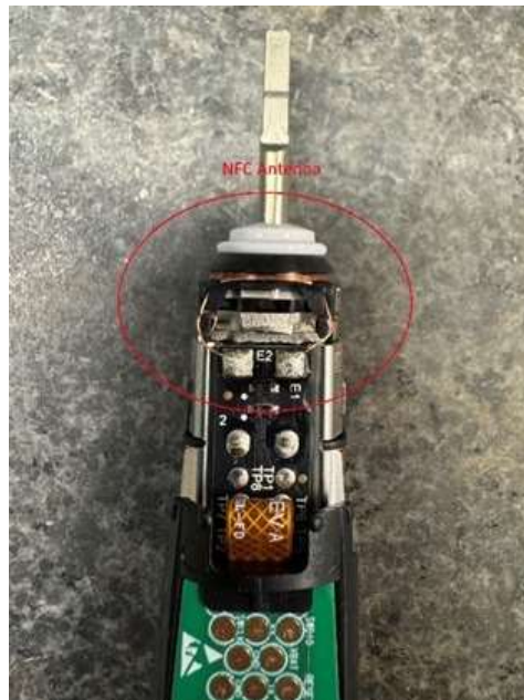
Figure 10: NFC Antenna on PCB2
