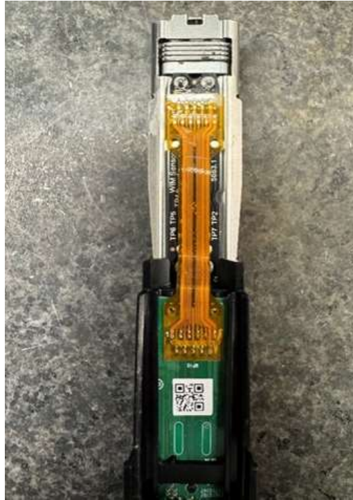
Figure 9: The flex PCB carries the NFC antenna traces from PCB1 to PCB2
