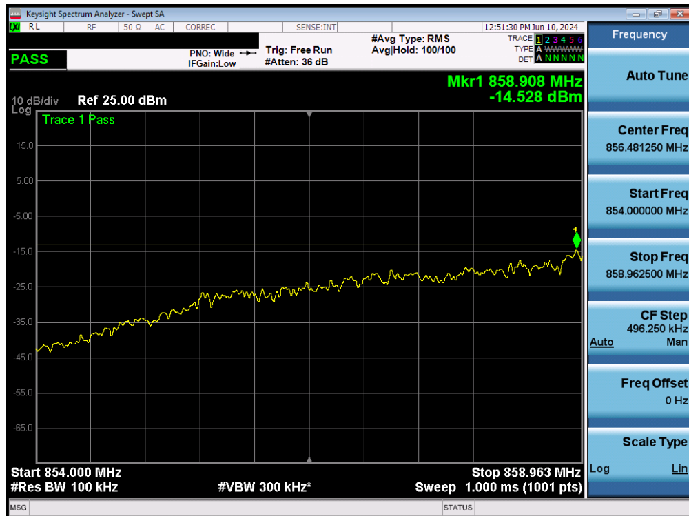
Plot 7-11. Lower Channel Edge Plot (LTE Band 26 - Low Channel)
