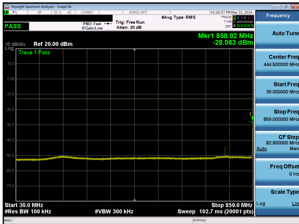
Plot 7-7. Conducted Spurious Plot (LTE Band 26 - High Channel)
