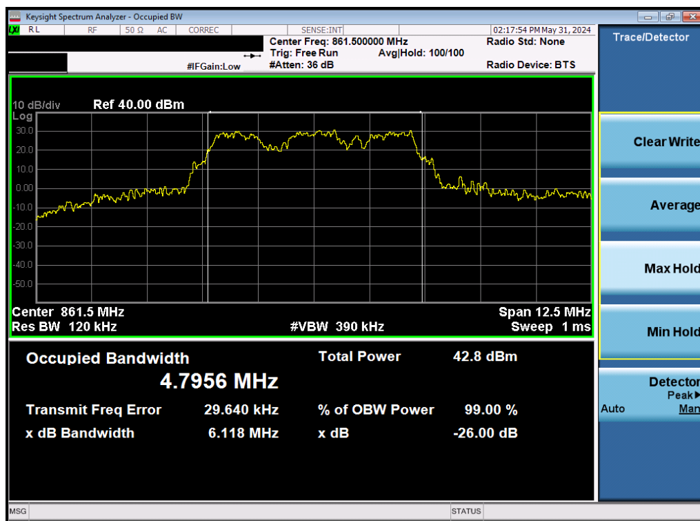
Plot 7-3. Occupied Bandwidth Plot (LTE Band 26)
