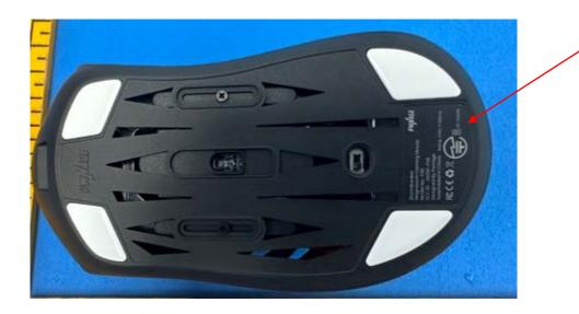
The label shown shall be permanently affixed at a conspicuous location on the device and be readily visible to the time purchase (Labeling requirements per 2.295)
