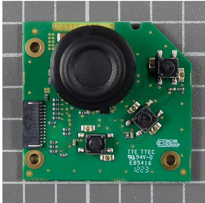
Wöhler VIS 700 – VIS 7 HD (monitor unit): Key PCB top view
