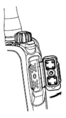
**Step 2** Align the accessory (such as audio accessory and programming cable) plug with the accessory connector.
