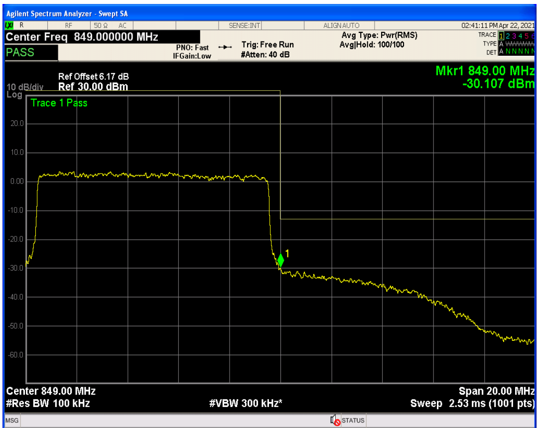
Band7 QPSK BW=5MHz Channel=20775 RB Size=1 Position=#0
