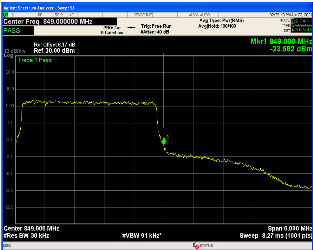
Band5 QPSK BW=5MHz Channel=20425 RB Size=1 Position=#Max
