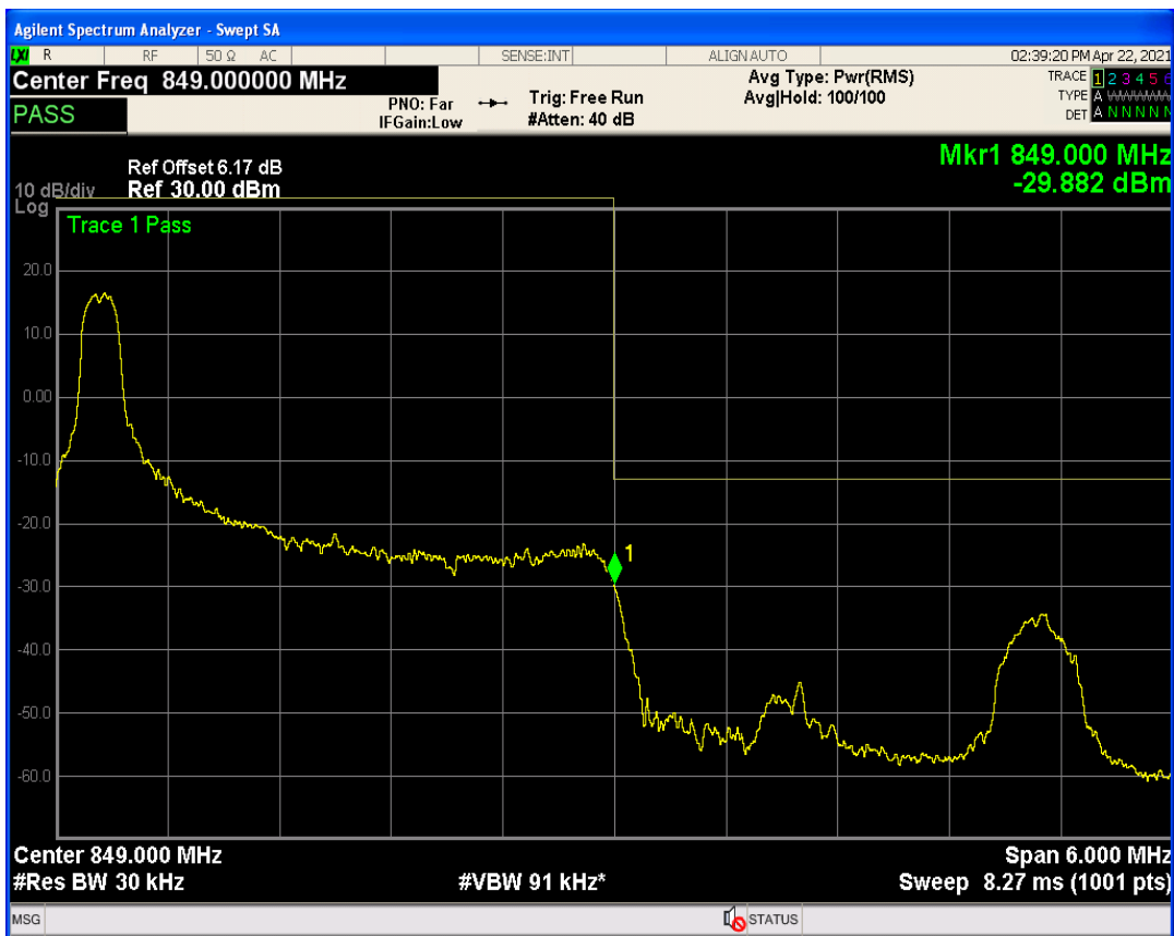
Band5 QAM16 BW=3MHz Channel=20415 RB Size=15 Position=#0
