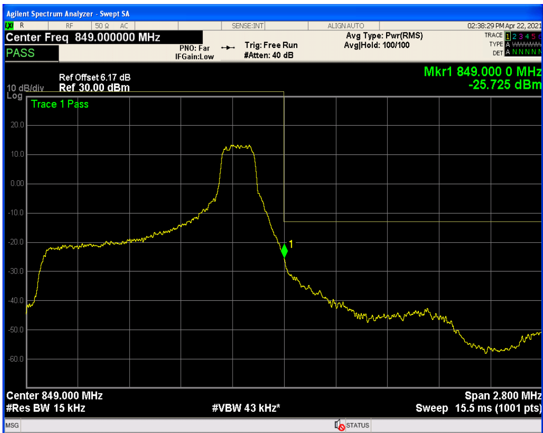
Band5 QPSK BW=1.4MHz Channel=20643 RB Size=6 Position=#0
