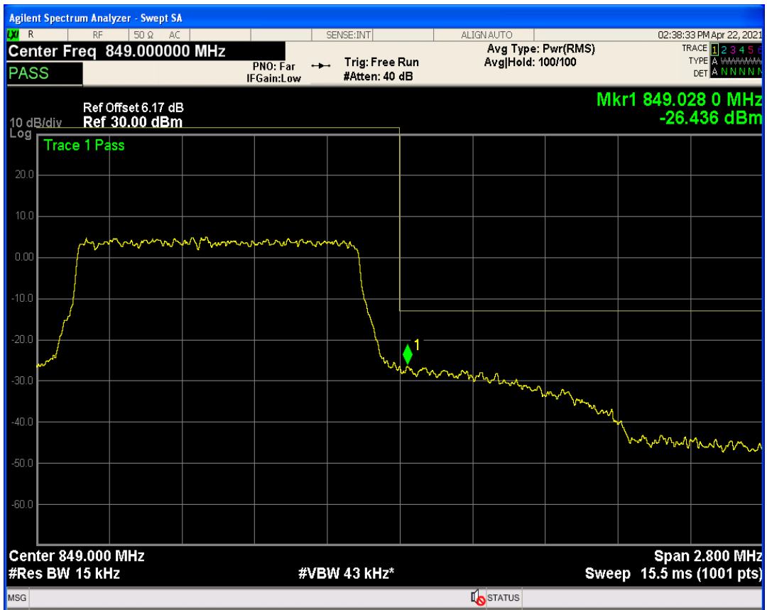
Band5 QAM16 BW=1.4MHz Channel=20643 RB Size=1 Position=#0
