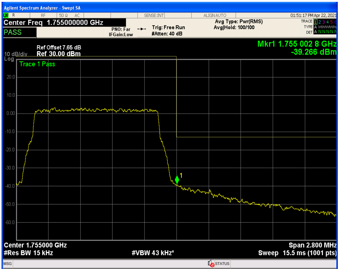
Band4 QAM16 BW=1.4MHz Channel=20393 RB Size=1 Position=#Max
