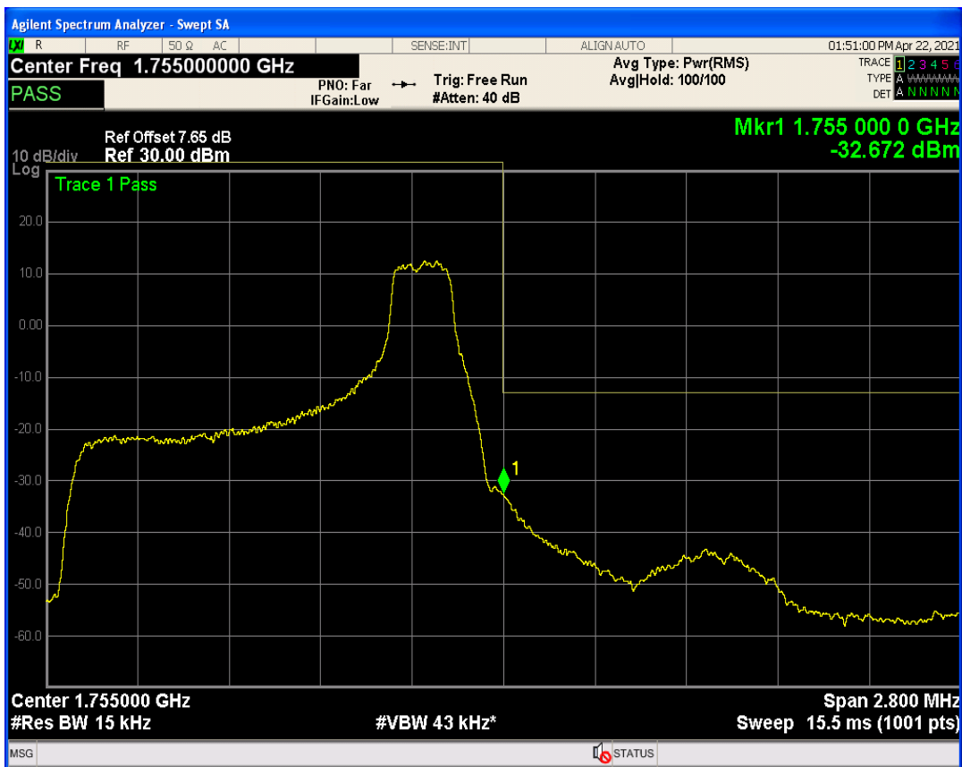
Band4 QPSK BW=1.4MHz Channel=20393 RB Size=6 Position=#0
