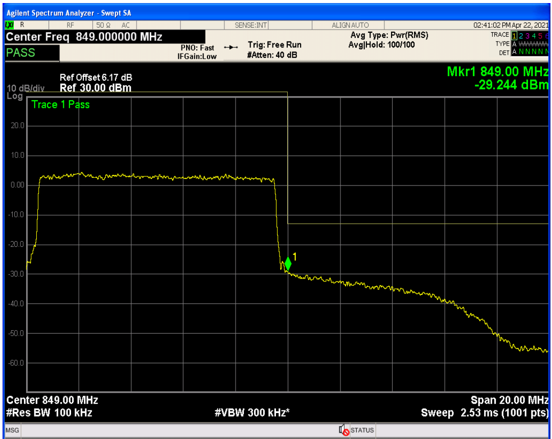
Band5 QAM16 BW=10MHz Channel=20600 RB Size=1 Position=#0
