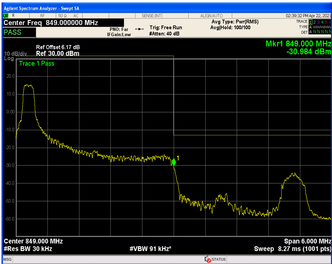
Band5 QAM16 BW=3MHz Channel=20635 RB Size=1 Position=#Max
