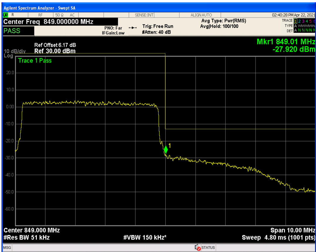
Band5 QAM16 BW=5MHz Channel=20625 RB Size=1 Position=#Max
