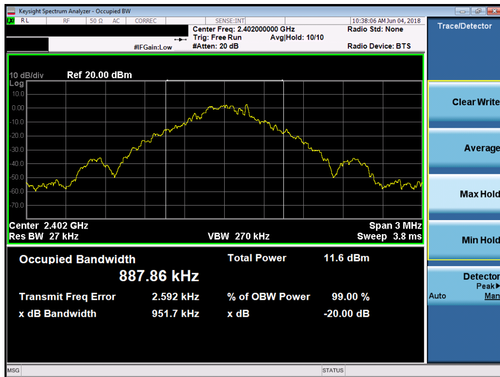
Plot 7-1. 20dB Bandwidth Plot (Bluetooth, 1Mbps – Ch. 0)
