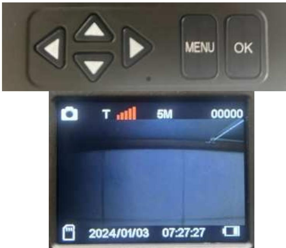
Menu button is for menu setting ,press the menu button, the camera will enter the menu setting interface (as shown below)
