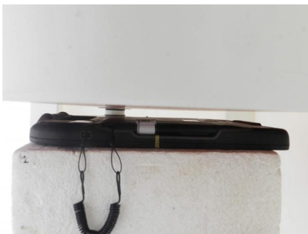
Bottom Face, Test Separation 10 mm
