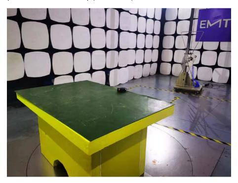
Spurious Emission Test Setup (Above 1GHz)
