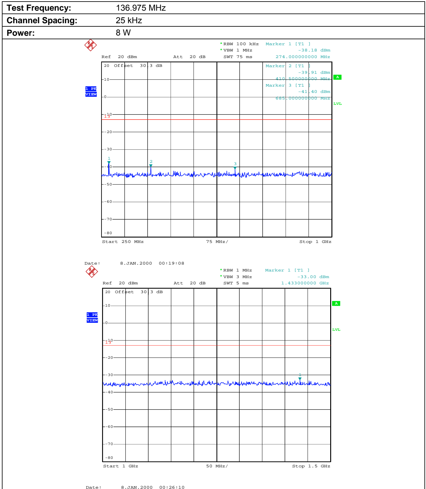
Plot 5.10.4.6. Conducted Transmitter Spurious Emissions 250 MHz – 1.5 GHz
