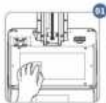
Peel off the protective film Clean the LCD screen
