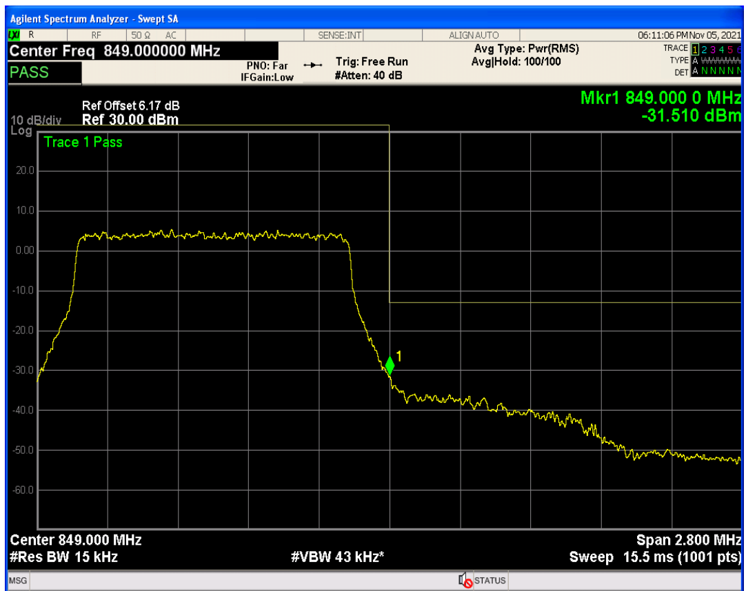
Band5 QAM16 BW=5MHz Channel=20425 RB Size=1 Position=#0
