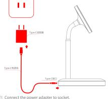
① Connect the power adapter to socket. ② Type-C cable one interface connected to the power adapter , the other interface to magnetic desktop wireless charger.
