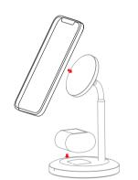
When the wireless charger is connected to an ordinary 5V adapter through Type-C to Type-C cable (Standard cable for this product) or USB-A to USB-C cable, the product works in ordinary wireless charging mode and only supports single 5W load. If you use QC , PD standard adapter, the product will works in quick wireless charging mode and supports 7.5W/10W/15W load.
