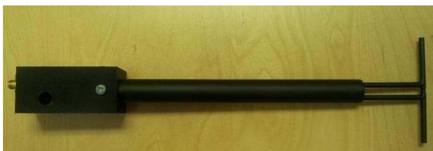
Figure 1 – MVG COMOSAR Validation Dipole
