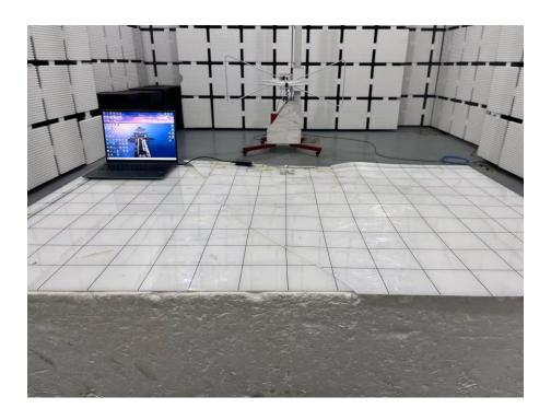
Set-up for Radiated Spurious Emission, Above 1GHz
