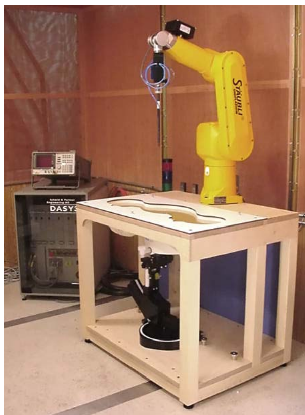
DASY3 SAR Measurement System with SAM phantom
