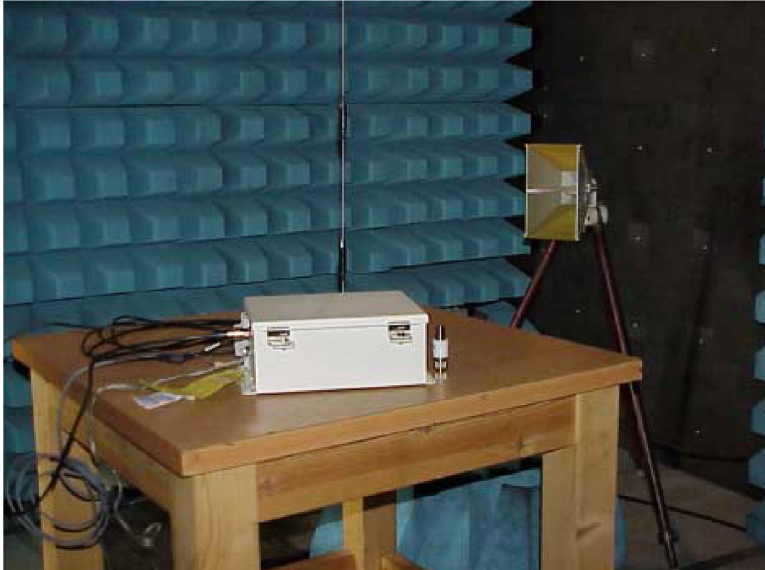
Photo 5. BreezeAccess SU-M-900 Spurious emission test setup in semi -anechoic chamber
