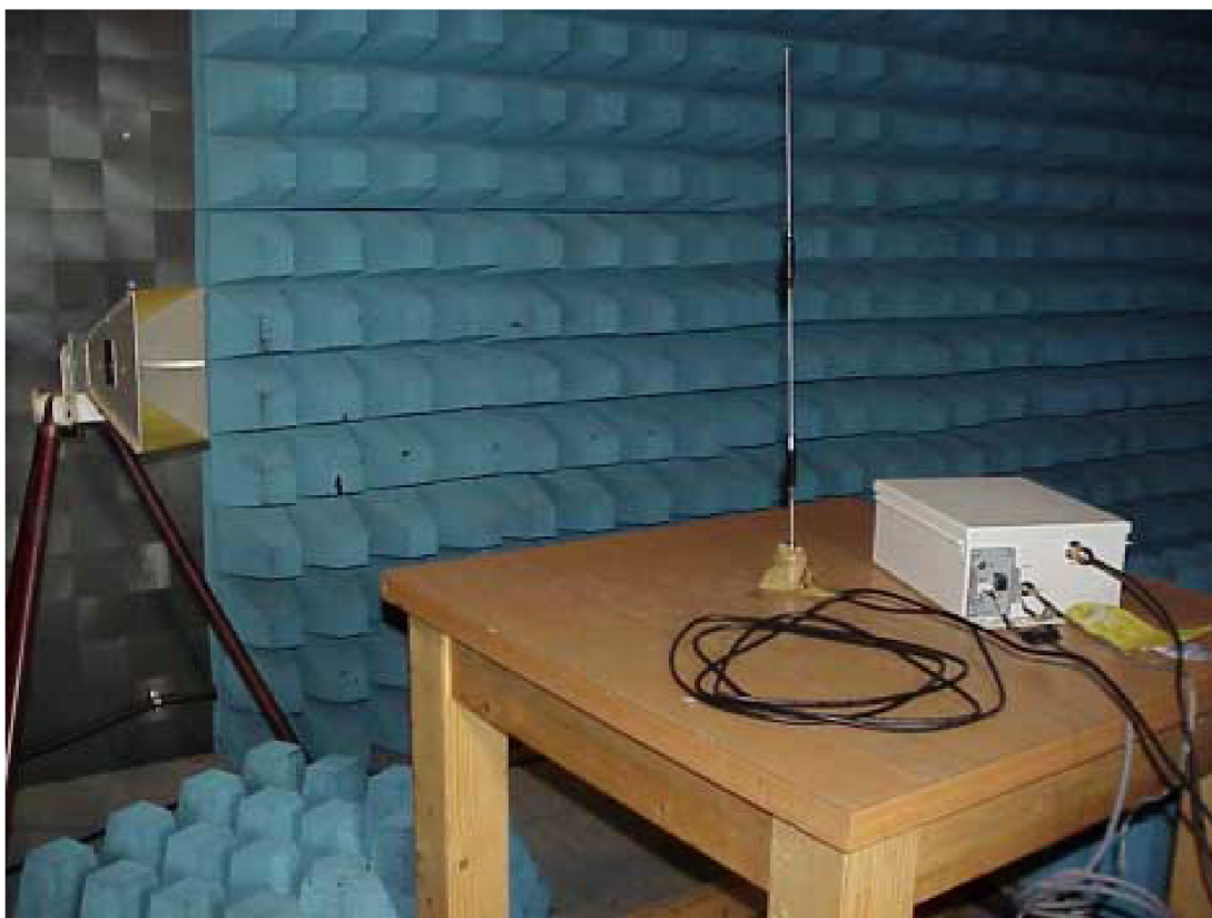
Photo 4. BreezeAccess SU-M-900 Spurious emission test setup in semi -anechoic chamber
