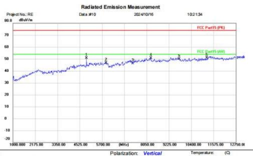
Site Limit: FCC Part15 (PK) EUT: Wireless Mouse M/N: Flow Mouse
