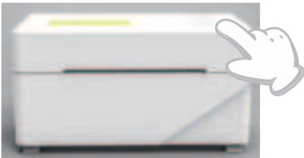
Since the printer needs to measure the length of the thermal paper, a stack of labels with at least 3 sheets is required to complete the process.
