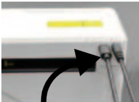
4. Turn the power ON (Press down "-" means Power ON), now you will see the light flashing!
