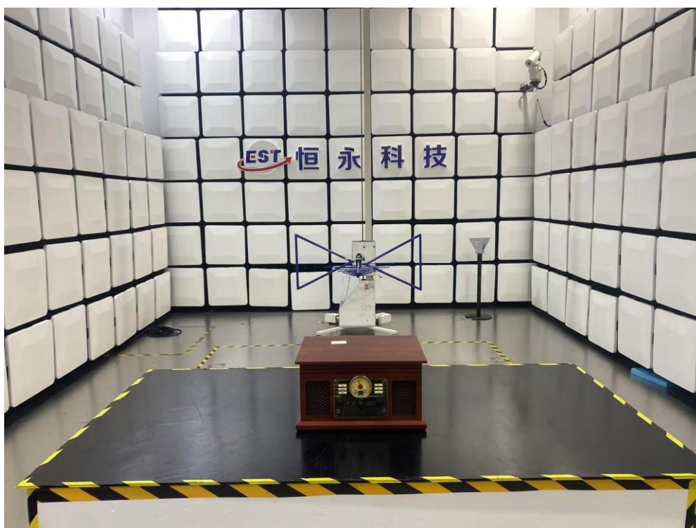
Radiated emission test: Below 1GHz
