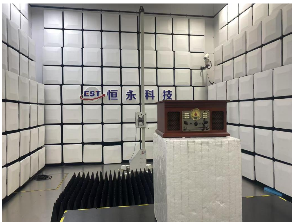
Radiated emission test: Above 1GHz
