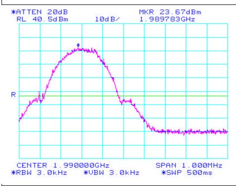
Notes: GSM-Tx single carrier 1989.8 MHz Power Reduced to comply with bandedge
