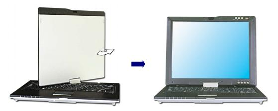
**3**. Adjust the slope of the display panel for comfortable viewing after making a rotation completely.
