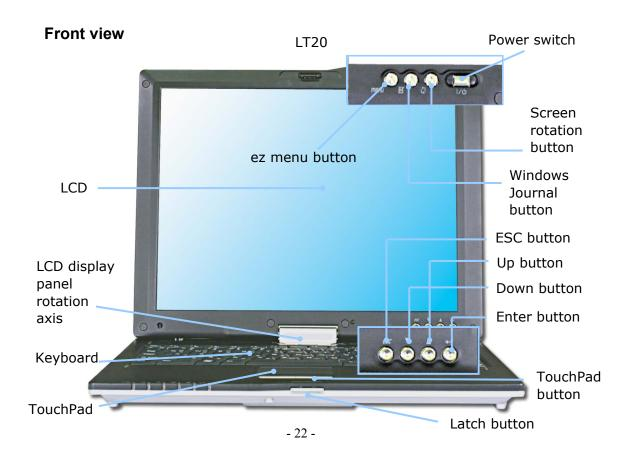
**Note:** ez menu button, Windows wordpad button, LCD rotation button, Power switch, Esc button, Up/Down button, and Enter button are coated for preventing static electricity purposes.
