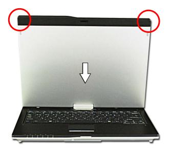
**5**. Fix the latch switch on LCD panel after folding as close to the keyboard completely.
