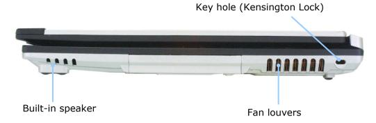
**Security key hole** (Kensington Lock): User can attach a separately purchased chain lock into the security keyhole and connect it to a fixed object to prevent a notebook theft.
