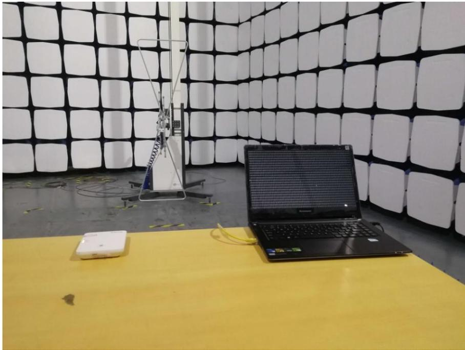
**FP - Radiated Emission test view (Frequency above 1GHz)**
