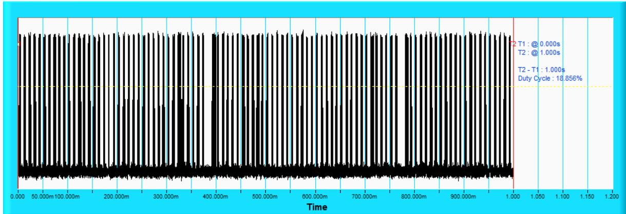
**NOTE:** T1 denotes the start of duty cycle period is 0th second. T2 denotes the end of duty cycle period is 1th second. T2 – T1= 1 seconds. Duty Cycle = 18.856%.
