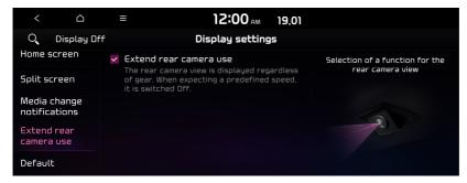
When you shift to "P" (Park) or drive at a predetermined spped or faster, the rear view display disappears to display the previous screen.
