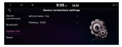
The passykey is a 4-digit authentication code used for a Bluetooth connection between the mobile phone and car system. The defauly passkey is set to 0000.
