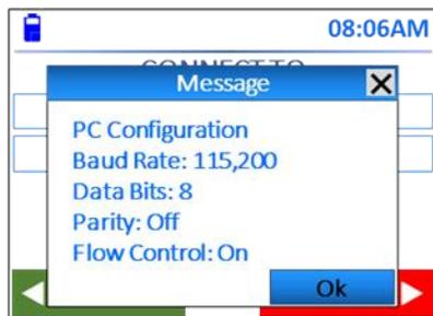
Open the GPScanID Software on your computer. The software is supplied on a USB drive with the reader or you can download the latest version of the software from:
