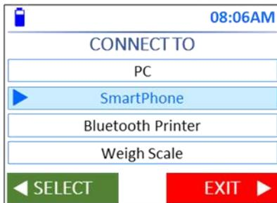
On the reader, go to **Settings > Connection > Bluetooth > SmartPhone** to set Bluetooth Connection parameters
