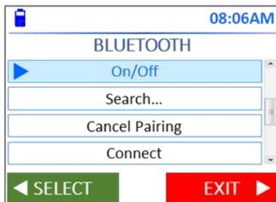
On the reader, go to **Bluetooth > On/Off** and select **On** to turn on the Bluetooth function
