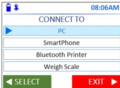
On the reader, go to **Settings > Connection > Bluetooth > PC** to set Bluetooth connection parameters
