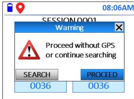
If Search is selected, the reader will continue to search for GPS signal for 60 seconds. User will have to wait in this period and ensure the reader is located in an open sky area. If the reader is still unable to get a lock on the GPS signal, the **No GPS Signal** warning appears again.
