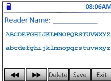
Use the **▲▼◀▶ Keys** to navigate between the rows and to the first character of the reader name then press the **MENU/OK button** to select. Repeat for each character of the name. Use the **◀▶** buttons to toggle between the alpha and numeric symbol input screens.
