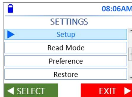
Use the ▲ / ▼ **keys** to navigate to **Setup** then press the ◀ **key** or **MENU/OK button** to select. The following Setup menu appears.
