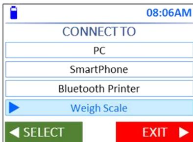
On the reader, go to **Settings > Connection > Bluetooth > Weigh Scale** to set Bluetooth Connection parameters
