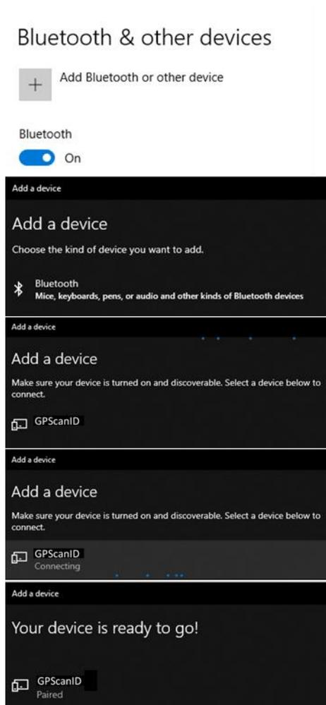
On the PC, go to Bluetooth settings and turn on the Bluetooth function. Then select **Add a Bluetooth device** and search for the reader. Once you have identified the Reader, **click on the reader details** to connect/pair with the reader. When connected the PC should identify the reader as being **paired**.
