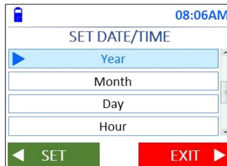
Use the **▲ / ▼ keys** to navigate to each input field and press the **◀ key** to select, then press **MENU/OK button** to save and exit the setting.
