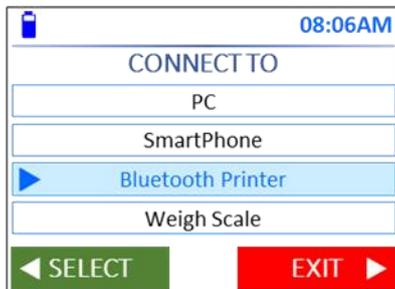
On the reader, go to **Settings > Connection > Bluetooth > Bluetooth Printer** to set Bluetooth Connection parameters
