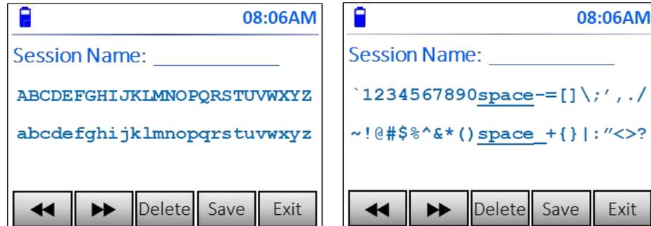
Use the ▲ ▼ ◀ ▶ **Keys** to navigate between the rows and to the first character of the session name then press the **MENU/OK button** to select. Repeat for each character of the name. Use the ◀◀ and ▶▶ buttons to toggle between the alpha and numeric symbol input screens.
