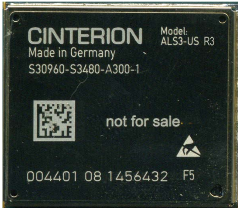
ALS3-US R3 label location lasing on shielding
