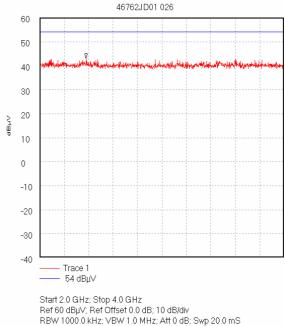
RBW 1000.0 kHz; VBW 1.0 MHz; Att 0 dB; Swp 20.0 mS Peak 2.38 GHz, 43.07 dBμV Display Line: 54 dBμV;; Limit Test Passed 02/12/2004 14:42:16
