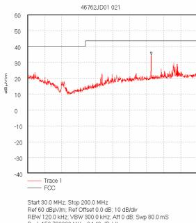
Peak 153.722222 MHz, 34.46 dBμV/m Limit/Mask: FCC; ; Limit Test Failed
