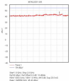
Peak 1.845556 GHz, 45.43 dBμV Display Line: 54 dBµV;; Limit Test Passed 02/12/2004 14:40:43
