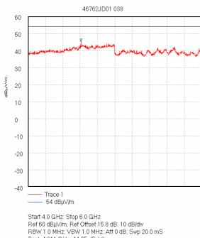
Peak 4.611 GHz, 44.85 dBµV/m Display Line: 54 dBμV/m; 09/12/2004 14:05:43
