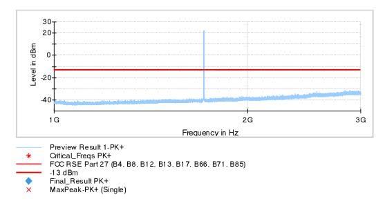
The peak above the limit is the carrier frequency.
