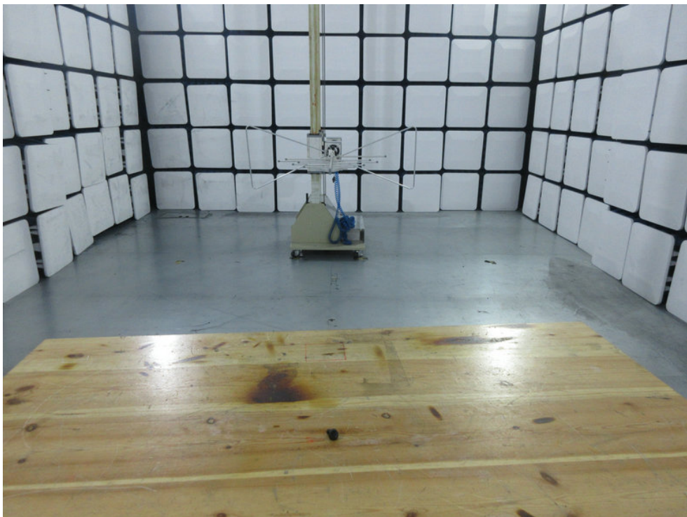
Photo of Radiation Emission Test
