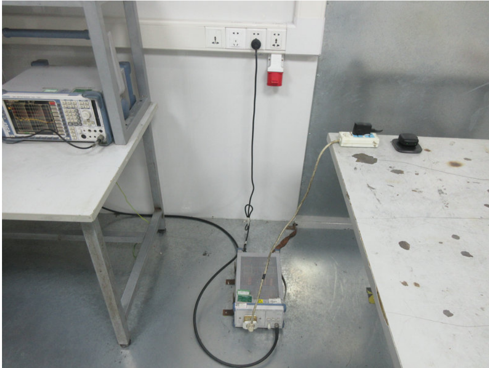
Photo of Conducted Emission Measurement
