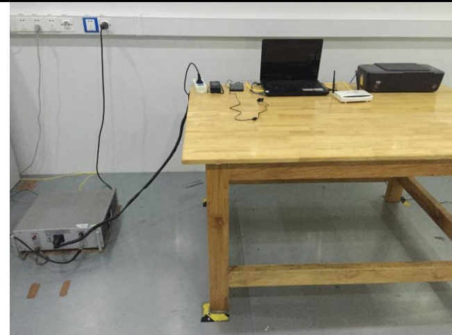
Conducted Emissions Test Setup – Front View
