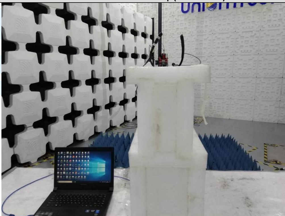
Radiated emission Test Setup (Above 1 GHz)
